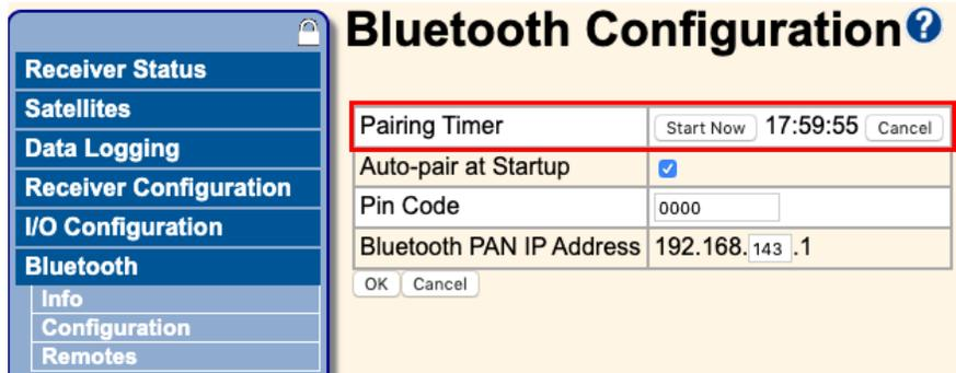
The timer can be also reinitiated without accessing the receiver WebUI by power cycling the receiver. While the timer is active, the *Bluetooth Info* menu will show that the module is discoverable.
