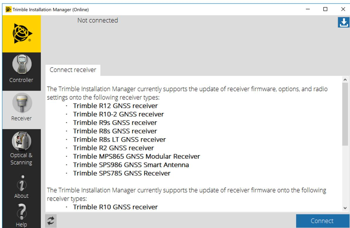
Trimble Installation Manager will display receiver-specific information. Select the firmware version you would like to install from the selection menu in the top right corner. Click on **Install** to start the installation process.
